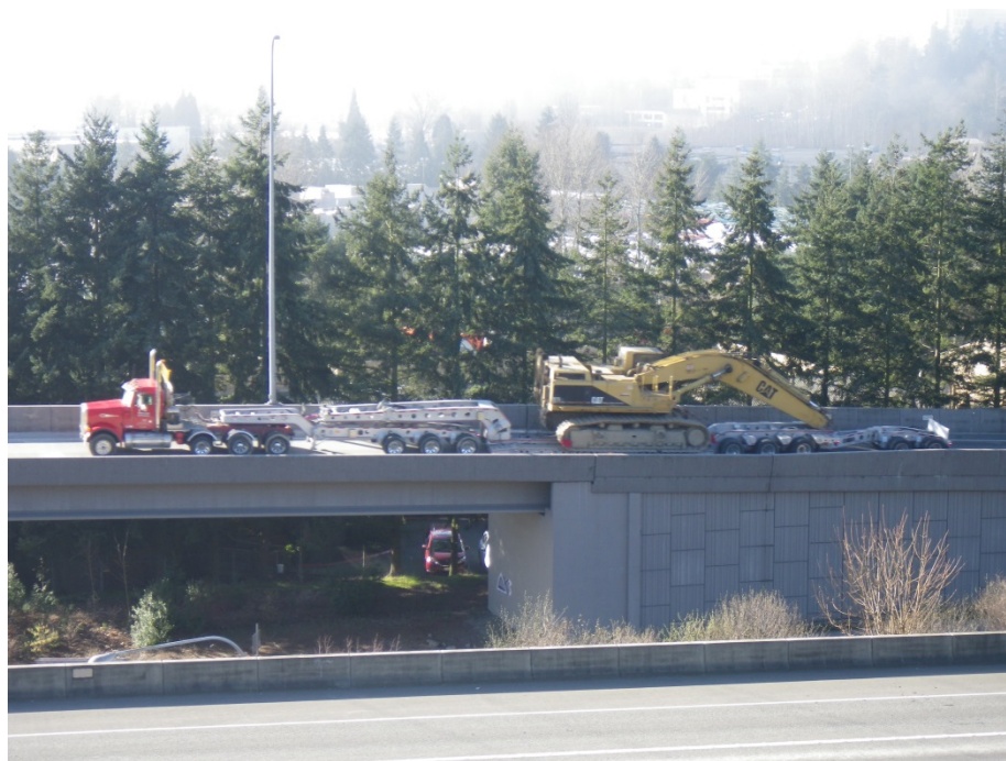
8-tire axles at 36 kips each
